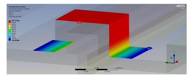
Fig 3(a) Surface Region #1: Width = 2.5 microns (centered over hottest part of channel)
