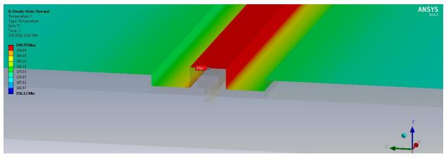
Figure 2(c): Surface temperature above the gate
