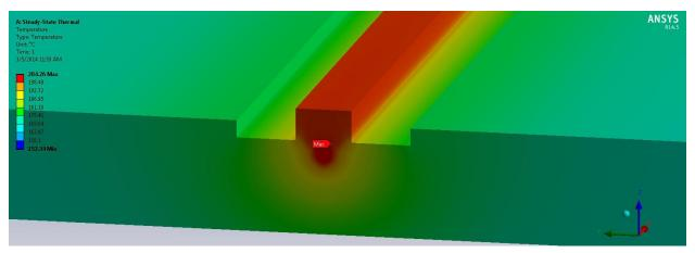
Figure 2(b):Temperature field in the ~2micron thick GaN layer above the SiC substrate
