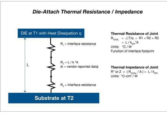
Figure 4: Illustration of die-attach thermal resistance / impedance
