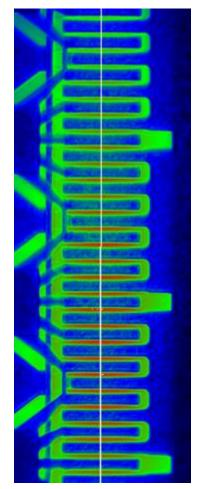
Figure 2: IR image of a typical GaN FET cell
