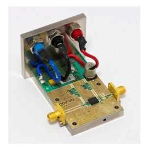
Figure 7: Photograph of the QPD1020 PA Reference Design
