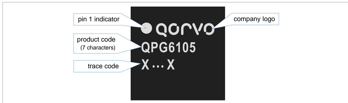
Figure 16: Information on the QFN32 Package
